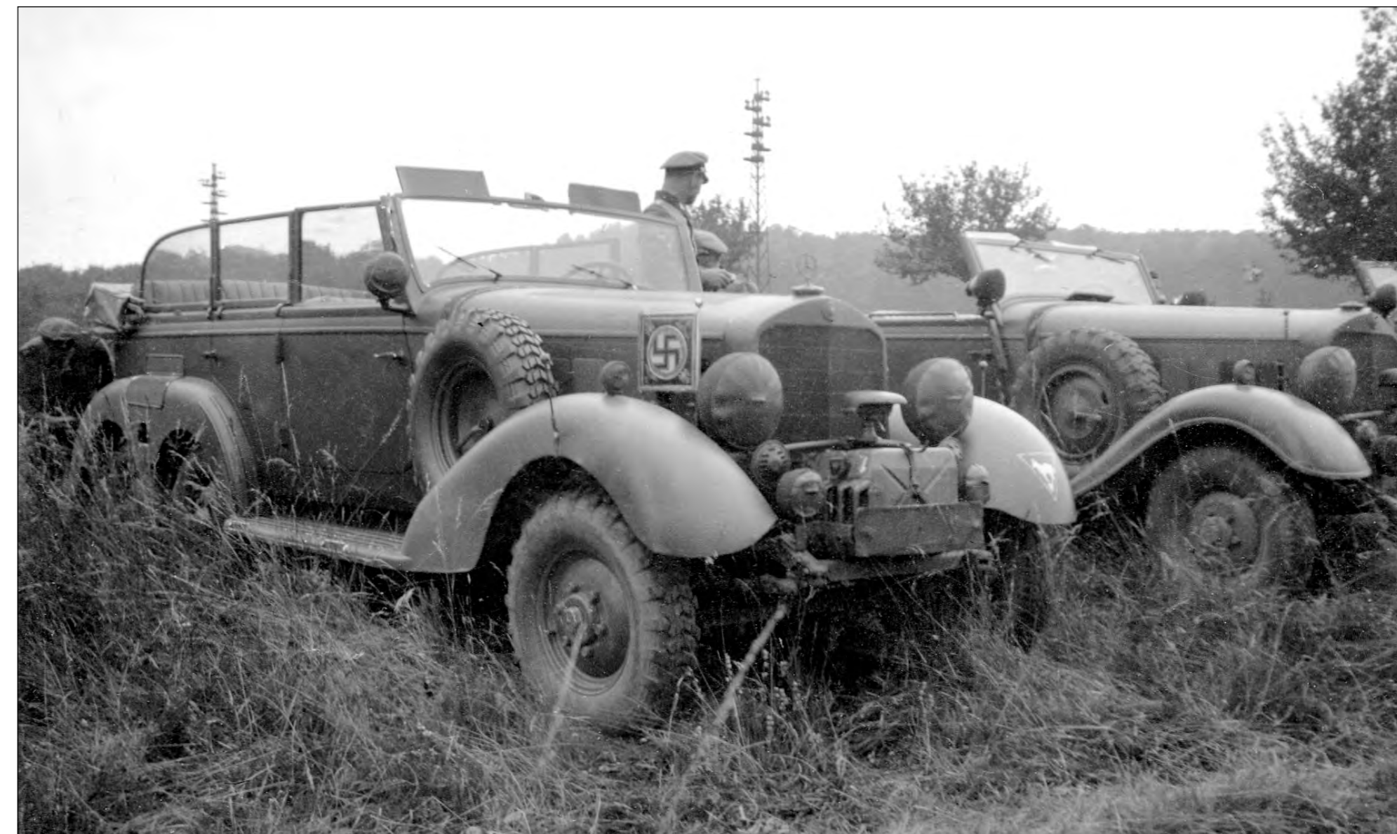
The G4 in the foreground is Hitler's, as indicated by the standard on the hood. Fuel cans can be seen secured in front of the radiator and the headlights are blacked-out to leave only a narrow beam of light. (K. Miller Collection).
