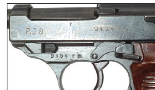
90. Side views and marking details on a Walther P 38
