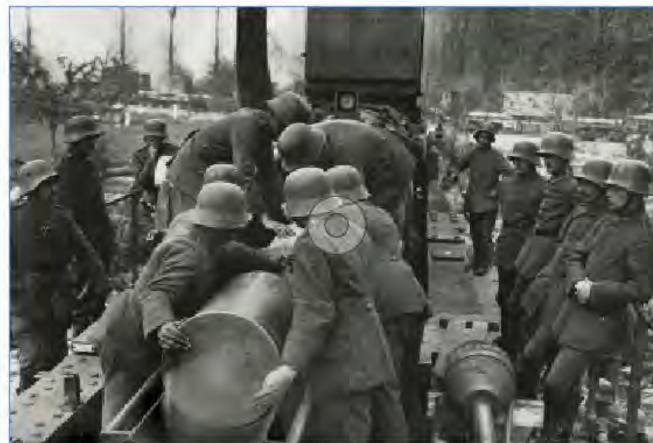
The high-powered artillery was formed by large-caliber guns and howitzers. In the photo, a group of artillerymen is about to load a 38 cm "SKL/45" gun, the largest caliber railroad artillery gun of the German Army. (Author's archive)
